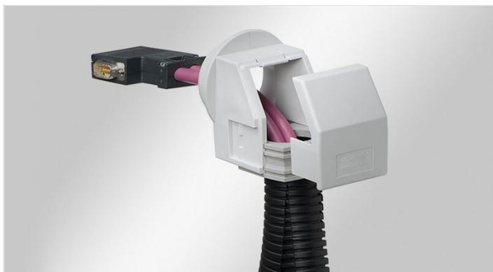
The split KVT-W90 cable glands are used to insert and seal pre-terminated cables at a 90° angle. But also electric, pneumatic or hydraulic lines without terminals or connectors as well as corrugated conduits can be easily routed (e.g. into control panels, enclosures or machinery) and sealed with IP54.
